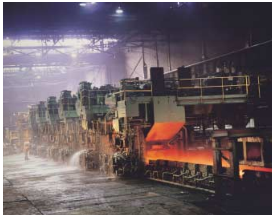
Reliability and serviceability are important factors in the design of high pressure systems. In this steel mill application, pump/motor sets (photo, top left) supply the lube system on the finishing stands of the strip mill. Rugged checkball pumps perform reliably even when subjected to extreme heat and contamination.
